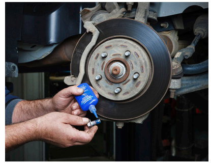
Permatex Medium Strength Threadlocker is strong enough to hold caliper abutment bracket bolts in place while the brake system is in operation but can easily be removed when the brakes need servicing.
