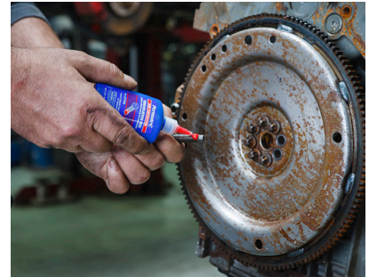
Permatex High Strength Threadlocker provides required holding strength in critical drivetrain applications.
