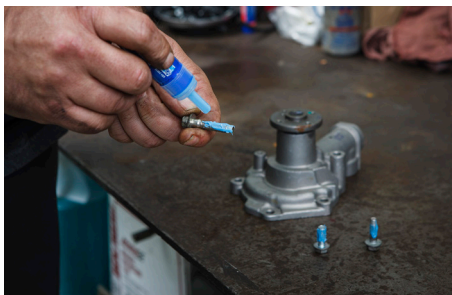
Permatex Medium Strength Threadlocker is ideal for locking and sealing water pump mounting bolts removed when the brakes need servicing.
